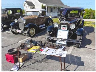
Also on display were a variety of parts including a distributor, coil, sparkplugs, head, piston and connecting rod, carburetor, intake and exhaust manifold, water pump and brake shoe assembly and drum. Students were able to handle the parts and they found the mechanical brakes compared to hydraulic brakes quite interesting.
